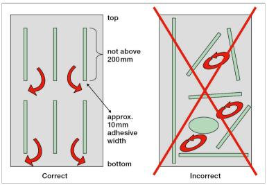
In order to avoid the confinement of the splitting product, a minimum space of 1,6 mm between mirror and substrate has to be kept mandatory. This space can be avoided most purposefully by sticking spacers onto the mirror. The minimum space specified serves the outbreathing of the splitting product. It does however not overrule the minimum distances for ventilation given by the Institute of Glass Manufacturing in Hadamar.
